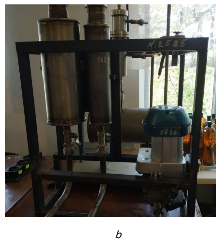
Fig. 1. Laboratory unit to study the impact of cavitation treatment on the ON and composition of gas-condensate gasoline with the addition of IPA: a – schematic of the unit ; b – a photograph of the unit ; T-1 – tank with raw materials (a mixture of GK-gasoline and IPA), T-2 – tank-separator for products, Cav – injector reactor that performs the cavitation treatment of raw materials, HPP – a high-pressure pump, Reg-1 – a three-way valve with control feature, Reg-2 – a three-way valve, PI – pressure gauge, FI – flow regulator
