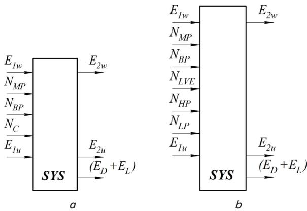
Fig. 4. The scheme of the exergetic transformations: *a* is the traditional heat pump installation; *b* is the LVE-based installation
