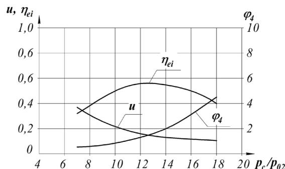
Fig. 1. The graph of the dependence of the degree of overproduction of steam  $\psi_4$ , the injection coefficient and the effective efficiency  $\eta_{ei}$  on the magnitude of the increase in the pressure of the passive flow  $p_c/p_{02}$  at  $t_{01}=121-149$  °C,  $p_{01}=300-500$  kPa, and  $p_{02}=5$  kPa
