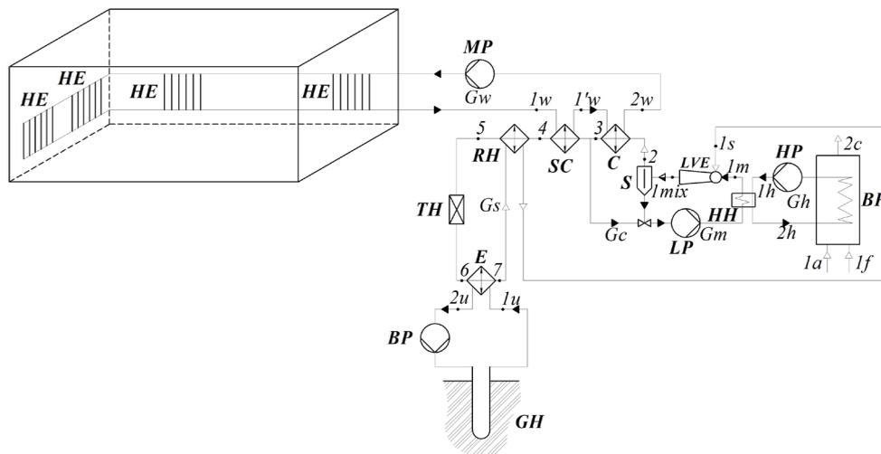
Fig. 2. The scheme of a heat pump based on a liquid-vapor ejector: LVE is the liquid-vapor ejector; S is the separator; LP is the liquid-vapor ejector circuit pump; HH is the heat subexchanger-heater; HP is the heat pump; HB is the boiler; C is the condenser; SC is the subcooler; RH is the regenerative heat exchanger; TH is the throttle device; E is the evaporator; BP is the brine pump; GH is the ground heat exchanger; MP is the mains water pump; HE is the heat exchanger
