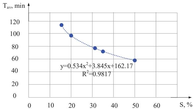
Fig. 9. Predicted time of failure  $T_{av}$  of a cutting insert made of hard alloy T15K6, depending on the area of shading in chemographic analysis
