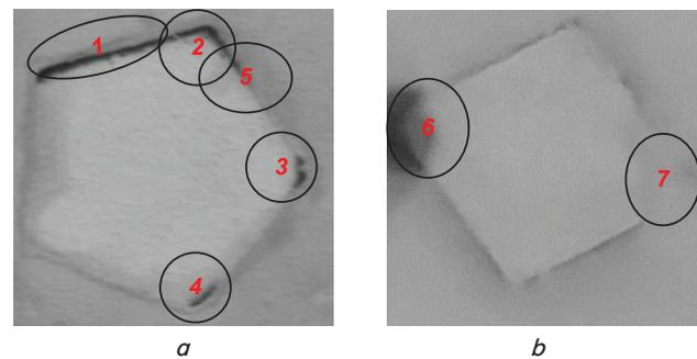
Fig. 4. Chemographic images of hard alloy plates: *a* – coated working edge; *b* – blackness degree in the images is associated with the defectiveness of the material and depends on the operating time of the plate
