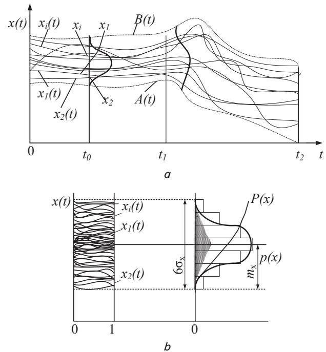
Fig. 1. An ensemble of realizations of a certain random process, defined in the same time interval: a – graphic interpretation of random values of the process  $x(t)$  in the section  $t$ ; b – statistical processing of the sample
