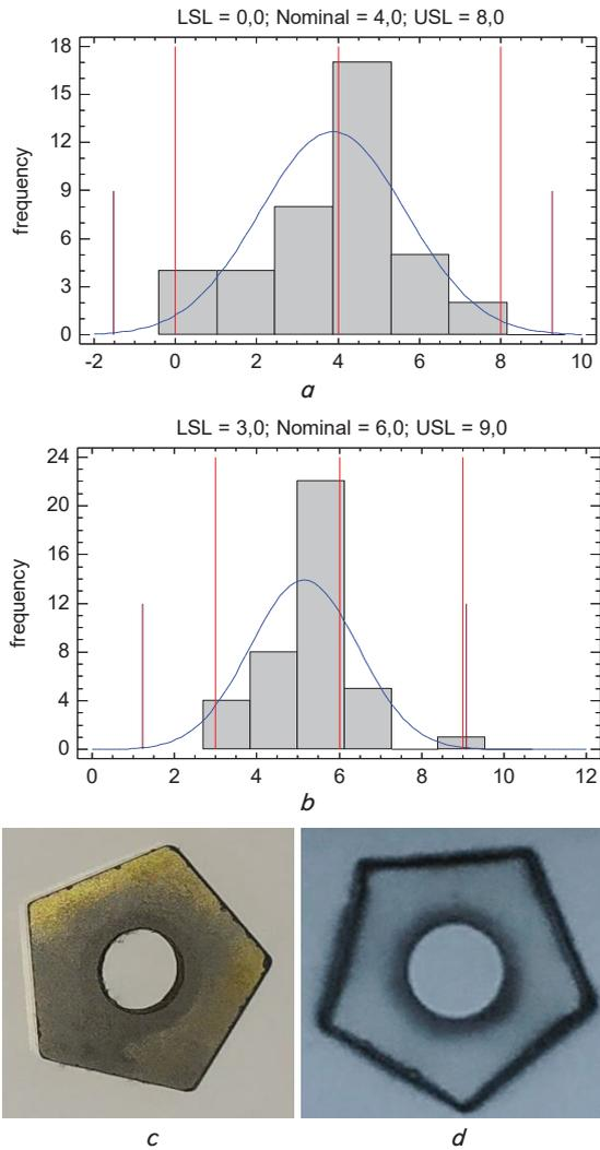
Fig. 5. Distribution of coating thickness and chemographic images of plates: *a*, *b* – distribution of coating thickness on the working surface of the plate; *c* – plate appearance; *d* – chemographic image of the working surface of the plate
