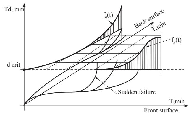
Fig. 3. Geometric interpretation of the onset of failure of an insert mounted on a cutting tool
