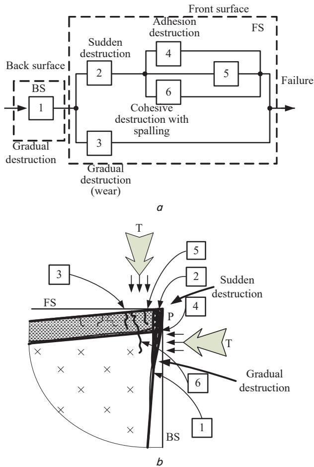
Fig. 2. Diagrams of damage manifestation and failure occurrence: *a* – damage to the front and back surfaces of the tool; *b* – scheme of failure manifestation
