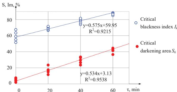
Fig. 8. Change in chemographic parameters depending on the loading time
