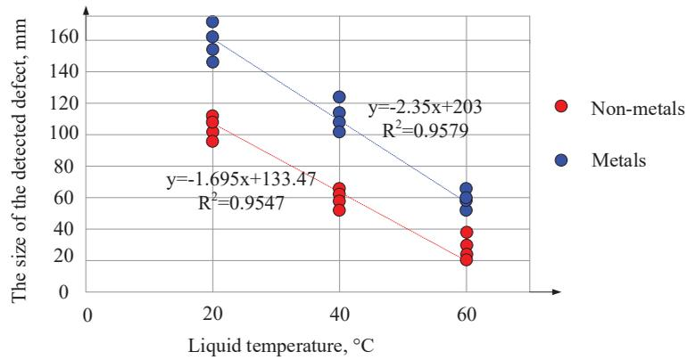
Fig. 7. Change in the size of detected defects depending on the temperature of the liquid
