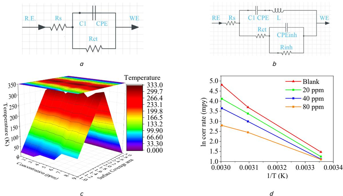
Fig. 3. Inhibitor effect in terms of: *a* – electrical equivalent circuit of white tea inhibitor one-time constant; *b* – electrical equivalent circuit of white tea inhibitor two-time constant; *c* – schematic 3D-surface coverage area of inhibition; *d* – corrosion rate of the mild steel with temperature variations
