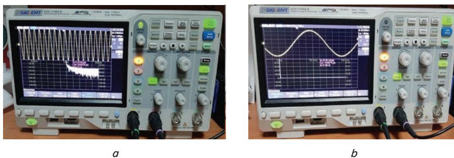
Fig. 17. Waveform of the output phase voltage of the frequency converter and its spectral analysis (fast Fourier transform): a – the load is a three-phase induction motor; b – the load is three wye-connected rheostats
