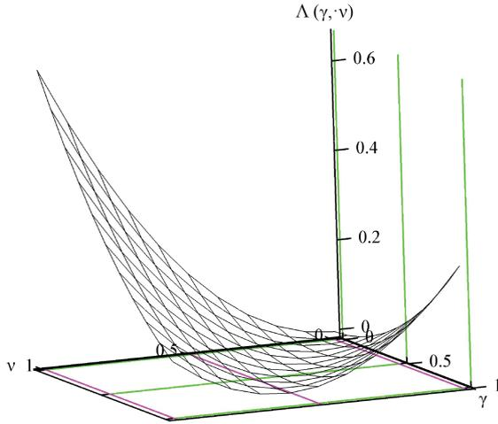
Fig. 6. Ratio of the orientation angles of a grinding machine headstock, which determines the minimum error of shape formation
