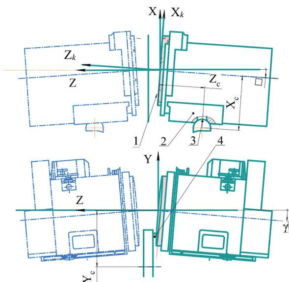
Fig. 1. Schematic adjusting of machine tool 3342 ADO for machining the ends of parts: 1 – grinding circle with a shape formation area; 2 – grinding machine headstock; 3 – spherical support; 4 – diamond pencil; 5 – drum to feed the parts with the place of installation of a diamond pencil; 6 – part
