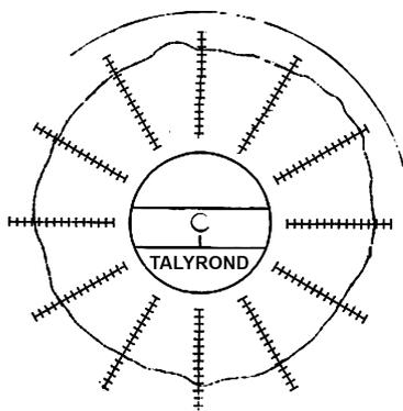
Fig. 4. Profilogram of the machined end surface
