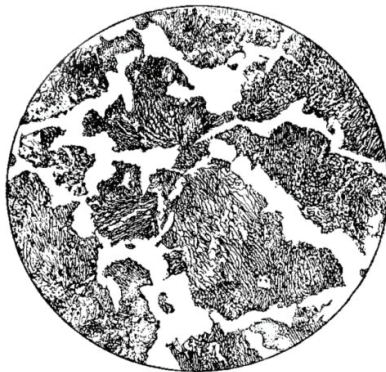
Fig. 4. The microstructure of steel 45 with sormite surfacing without hardening, \times 500 [16]
