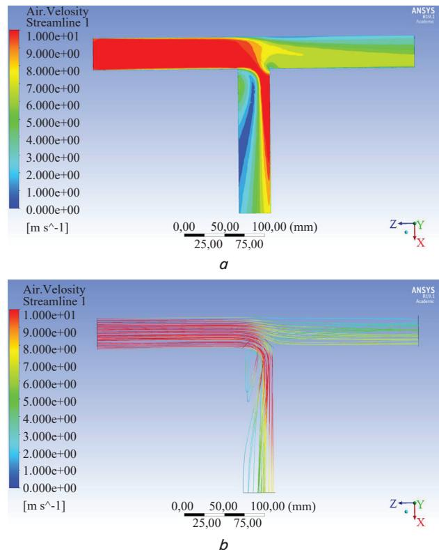
Fig. 3. Results of the refined calculation of the flow of air in a branching channel at angle 90°:  $a$  – the field of flow velocities,  $b$  – the flow streamlines
