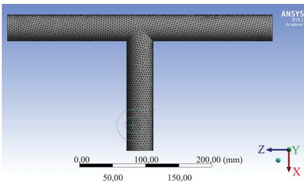
Fig. 2. The finite-volume model of the flow area with a side outlet at 90°
