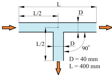
Fig. 1. The geometry of a channel with a side outlet at angle 90° – the length  $L$  and the diameter  $D$  are assigned
