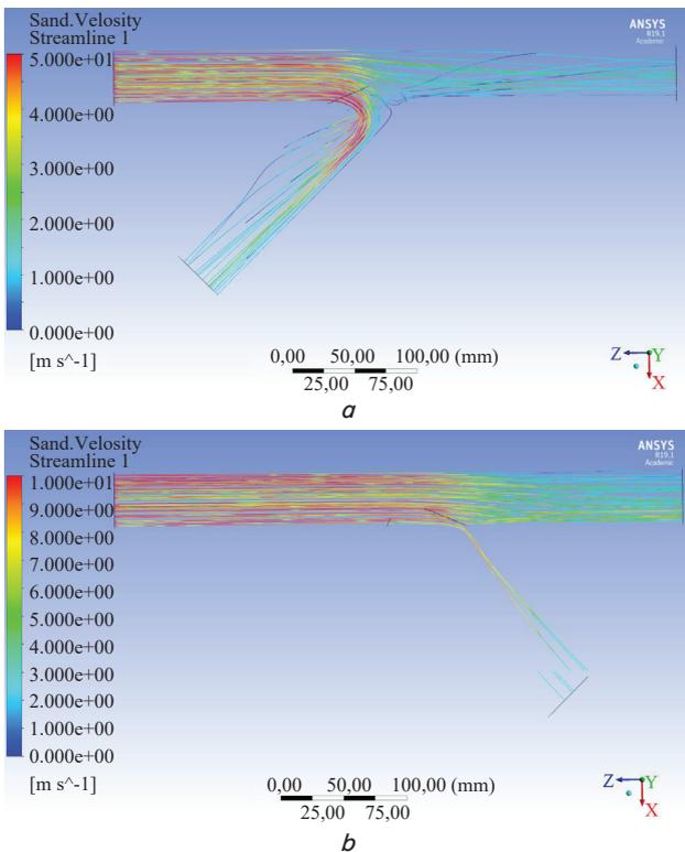
Fig. 7. Dust particle flow lines in a channel with outlets at different air velocity and particle sizes:  $a - 135^\circ$ ,  $d = 5 \mu\text{m}$ ,  $v = 5 \text{ m/s}$ ;  $b - 45^\circ$ ,  $d = 30 \mu\text{m}$ ,  $v = 15 \text{ m/s}$
