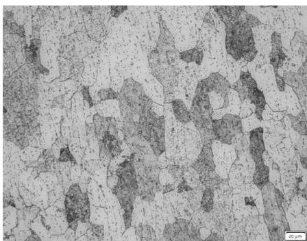
Fig. 1. Raw material of AISI 430 SS: *a* – x-ray diffraction pattern; *b* – optical micrograph. Aqua regia etchant
