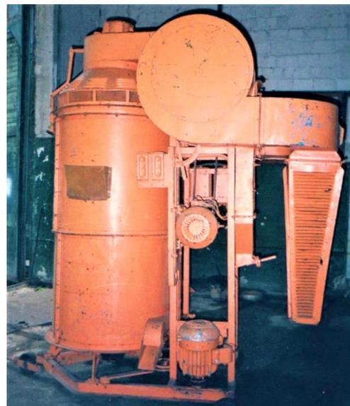
Fig. 1. General view of a pneumatic vibratory centrifugal separator
