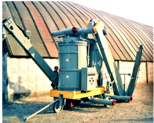
Fig. 3. General view of the modified self-sliding pneumatic vibratory centrifugal separator A1-BCS-100
