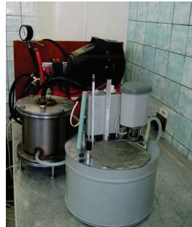
Fig. 2. General view of the setup for studying the beer microfiltration process [20]
