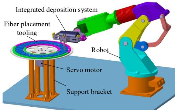
Fig. 7. Conceptual design of the robotic filament winding equipment
