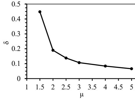
Fig. 5. Variation of unit mass stiffness against the radius ratio  $\mu$
