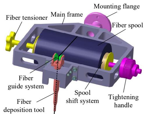
Fig. 10. The structure of the integrated deposition system
