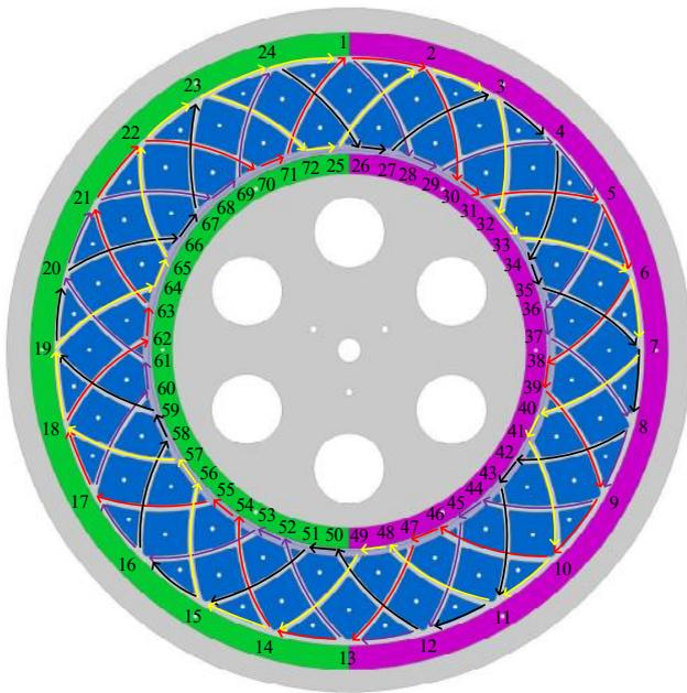
Fig. 11. The scheme of the winding trajectories
