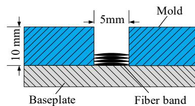
Fig. 9. Schematic of fiber placement inside the rib groove
