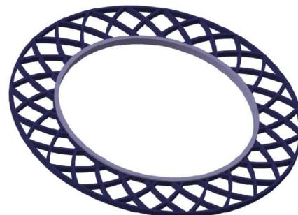
Fig. 12. The 3D model of the final component of the composite lattice ring structure
