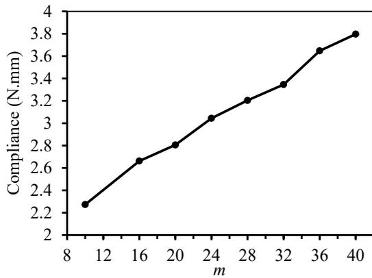
Fig. 3. Variation of structural compliance with the number of substructures,  $m$
