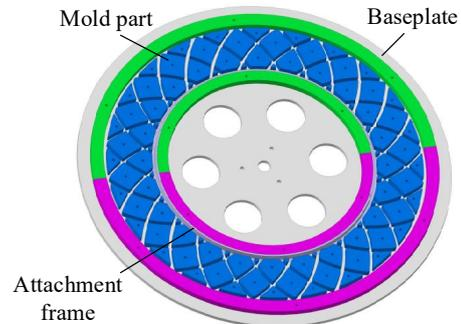
Fig. 8. Conceptual design of fiber displacement tooling
