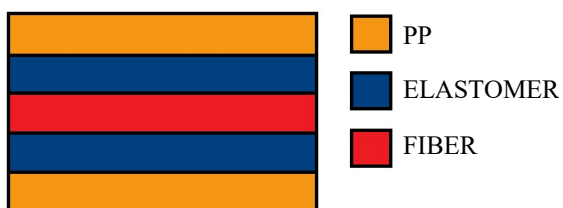
Fig. 5. Composite layout of sugar palm fiber-reinforced polypropylene-elastomer
