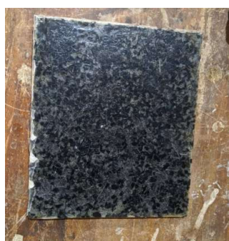
Fig. 6. Composite molding of sugar palm fiber-reinforced polypropylene-elastomer
