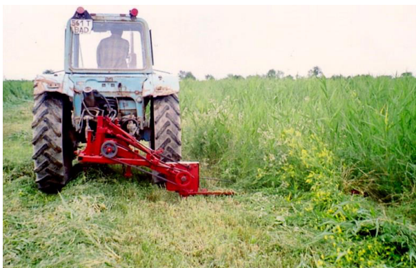
Fig. 10. KS-2.1M mower (modified high-speed mower) in operation, mowing forbs
