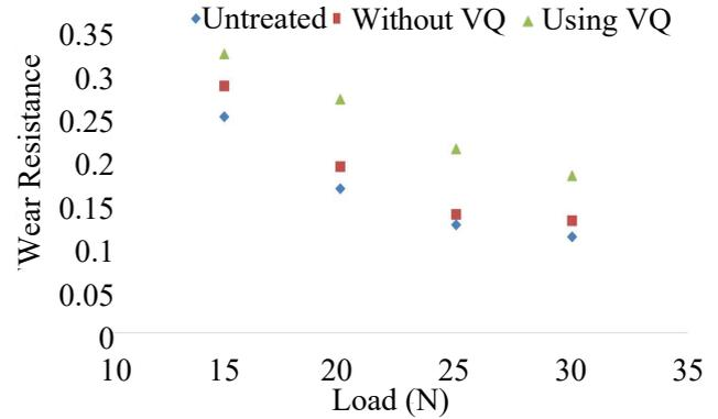
Fig. 5. Effect of vibrator quenching on the wear resistance of the specimen after pack carburizing treatment at optimum conditions
