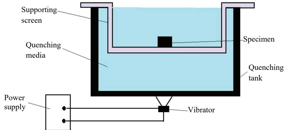
Fig. 1. Basic principle of vibrator quenching
