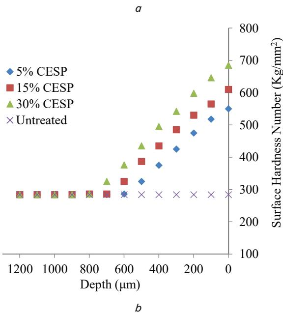
Fig. 4. Effect of carburizing agent on the surface hardness of the specimen: *a* – quenching without vibrator; *b* – quenching with vibrator
