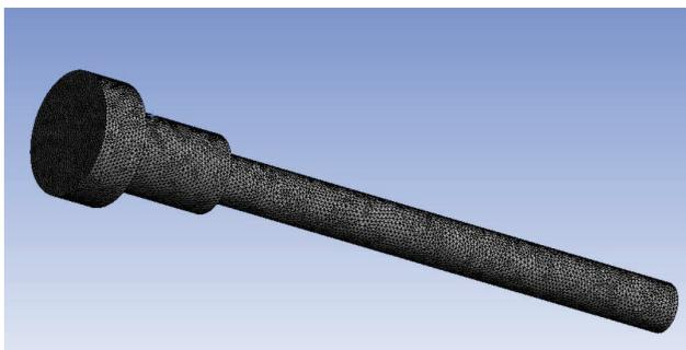
Fig. 3. Mesh image of the moving die
