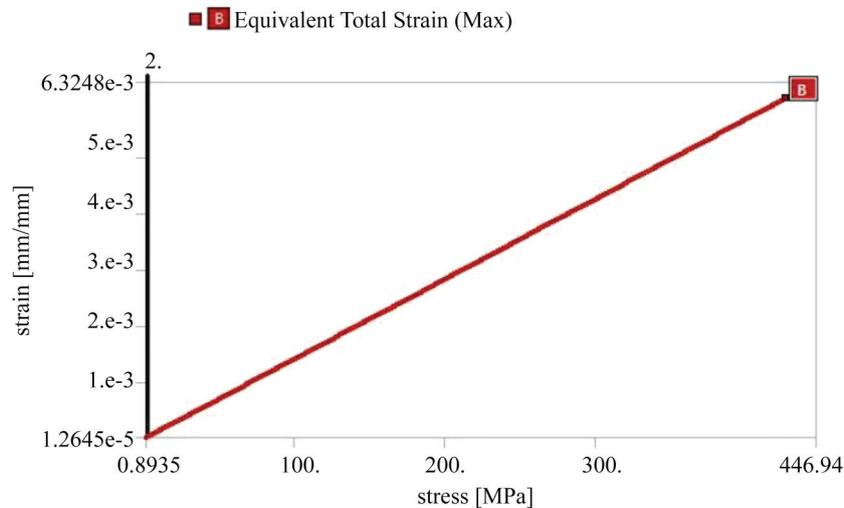
Fig. 7. Stress-strain relationship for aluminum alloy
