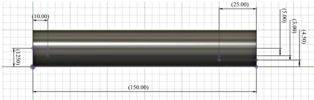
Fig. 1. 3D dimensional design of the fixed die
