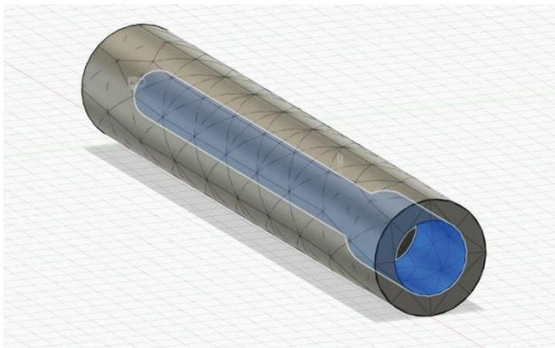
Fig. 2. Mesh image of the fixed die
