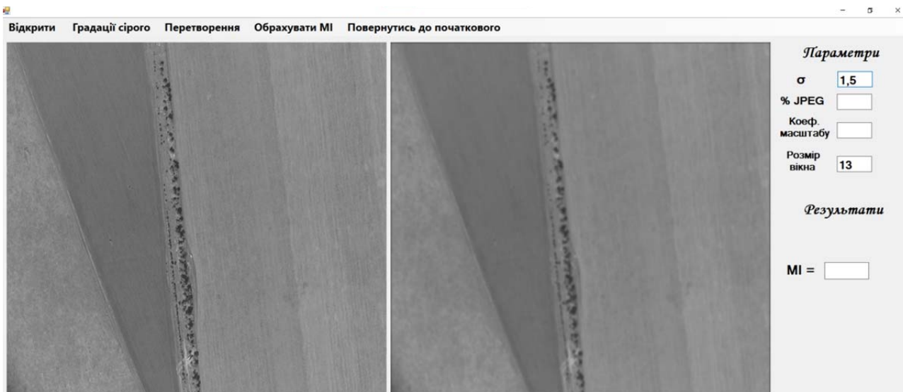
Fig. 5. Using the Gauss filtering method with parameter \sigma=1.5
