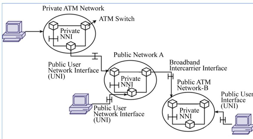
Fig. 1. The architecture of ATM Network Interface
