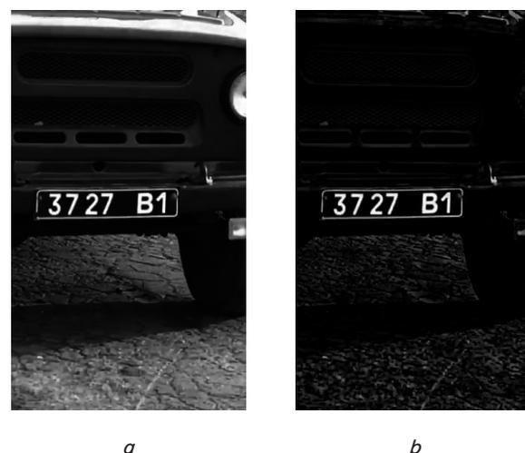
Fig. 4. Results of preliminary processing of the original image (Fig. 3): *a* - the result of the pixel-to-pixel multiplication of channels in the RGB color space; *b* - the result of using the morphological operation  $imtophat$
