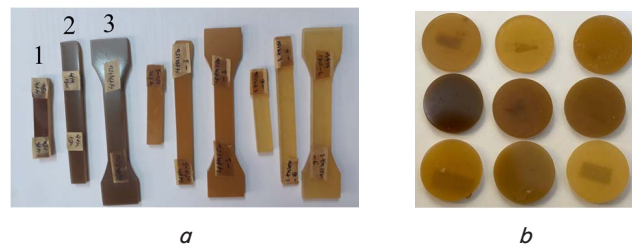
Fig. 3. Types of specimens used in practical tests: a – 1 impact, 2 flexural, 3 tensile; b – thermal conductivity
