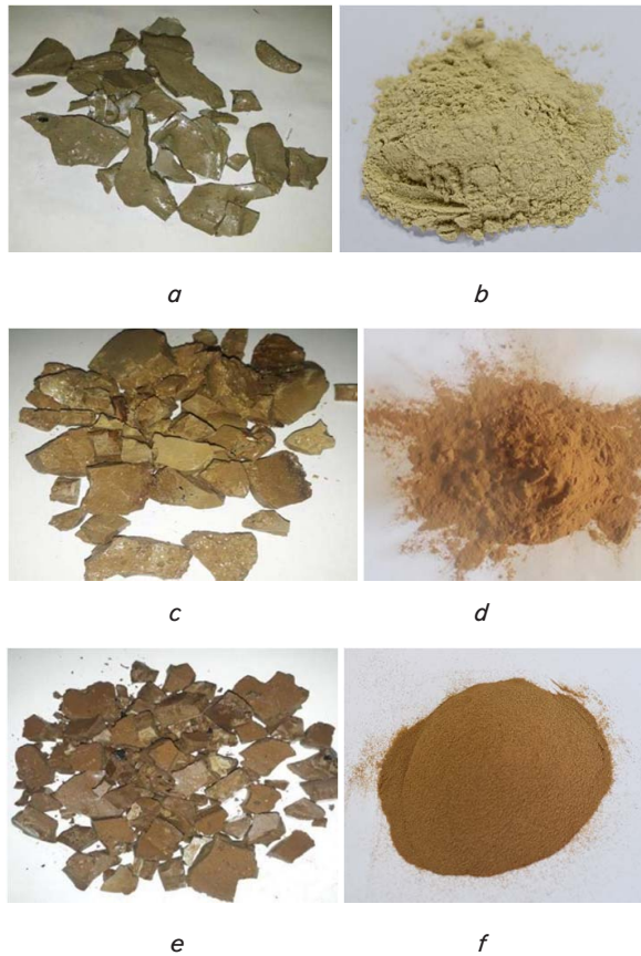
Fig. 2. The form of a melt of recycled waste after cooling and RCCF 75 μm at different heating time: a, b – 2 min; c, d – 4 min; e, f – 6 min
