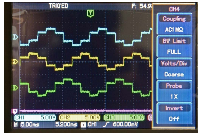
Fig. 14. Waveform of phase voltages of a three-phase inverter
