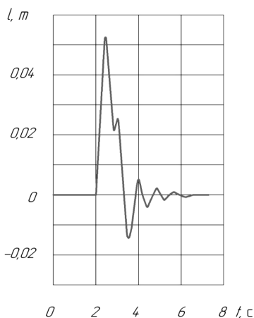
Fig. 6 Oscillogram of natural vibrations of the mass of the body on air suspension with balloon PS: (V_A/V_1)=0.7
