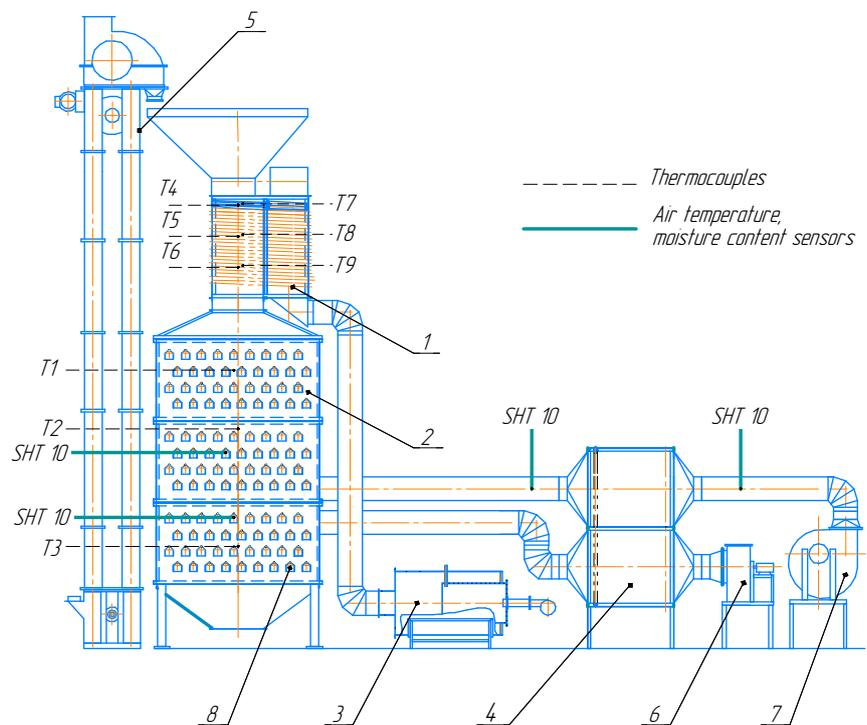
Fig. 2. Structure of the grain dryer based on thermosiphons: 1 – layer heater; 2 – drying chamber; 3 – heat generator; 4 – heater; 5 – noria; 6 – fan; 7 – fan, 8 – box
