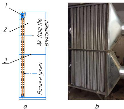
Fig. 4. Thermosiphon heater structure: *a* – diagram; *b* – photograph; 1 – finned thermosiphon; 2 – body; 3 – dividing wall
