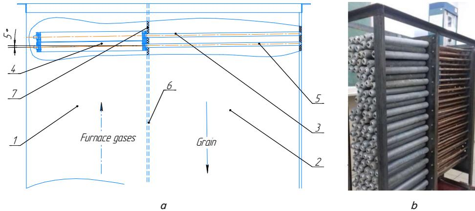
Fig. 3. Structure of the layer heater: *a* – diagram; *b* – photograph; 1 – gas duct; 2 – grain heating chamber; 3 – thermosiphon; 4 – evaporation area; 5 – condensing section; 6 – dividing wall; 7 – thermal insulation
