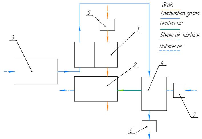
Fig. 1. Diagram of a grain dryer based on thermosiphons: 1 – layer heater; 2 – drying chamber; 3 – heat generator; 4 – heater; 5 – noria; 6 – fan; 7 – fan
