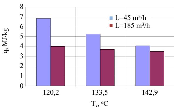
Fig. 10. Specific energy consumption of the dryer
