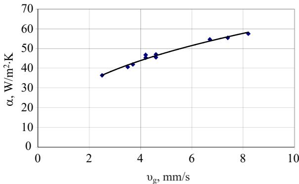
Fig. 5. Effect of average grain flow rate on heat transfer coefficient
