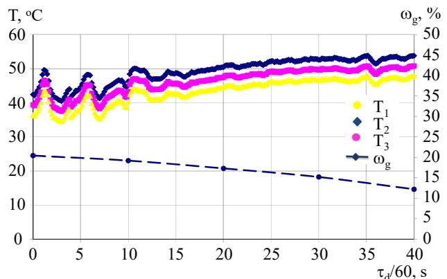
Fig. 7. Thermograms, drying curves at  $L=185$  m<sup>3</sup>/h
