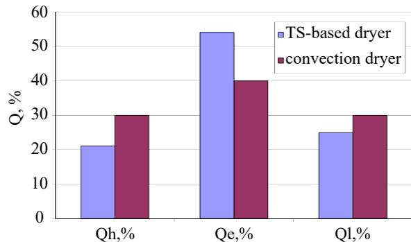
Fig. 11. Distribution of thermal energy in grain dryers
