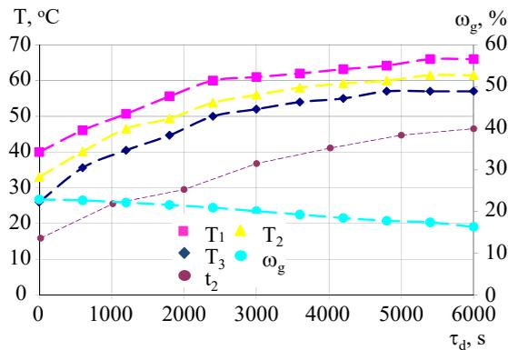
Fig. 9. Drying curves and thermograms of wheat grain  $G_w=550$  kg/h:  $T_1, T_2, T_3, ^{\circ}\text{C}$  – grain flow temperature;  $t_2, ^{\circ}\text{C}$  – air temperature at the outlet of the dryer;  $\omega_g$  – grain moisture content
