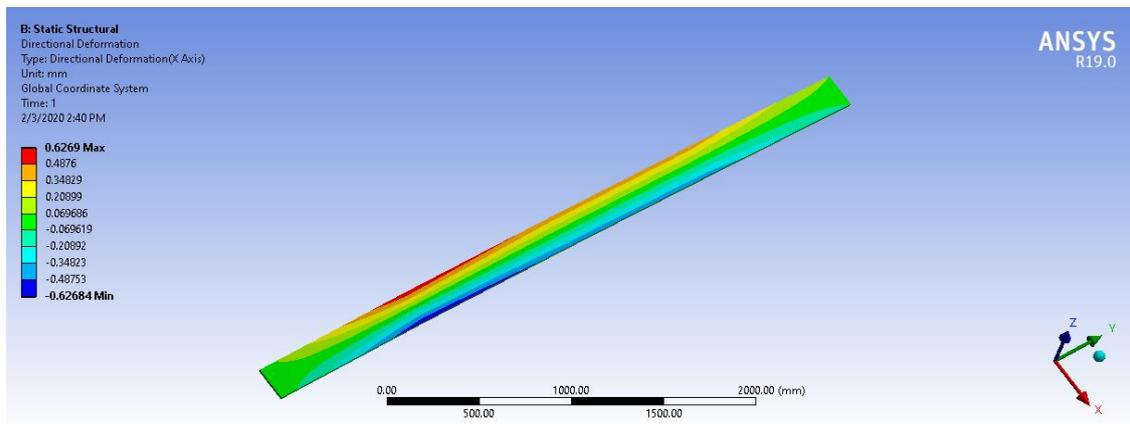
Fig. 4. Effect of the X-directional deformation
