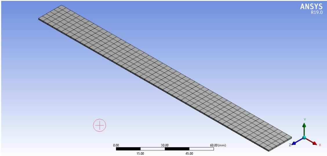
Fig. 1. Geometry and mesh of the cantilever structure
