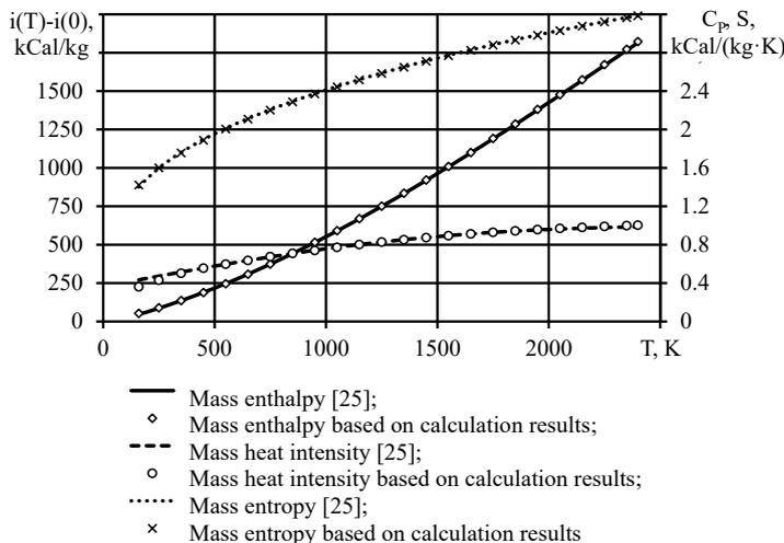
Fig. 3. Thermodynamic properties of pure kerosene combustion products depending on temperature
