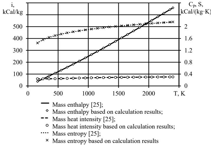
Fig. 2. Thermodynamic properties of dry air depending on temperature
