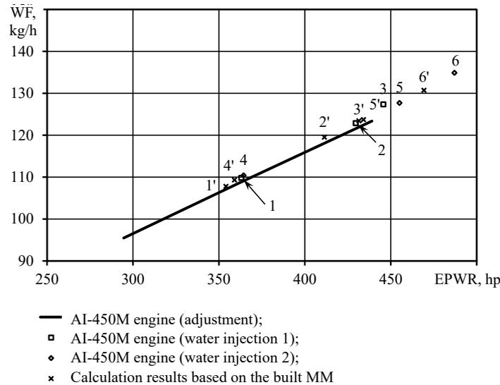
Fig. 5. Change in fuel consumption (WF) depending on engine operating mode and water injection
