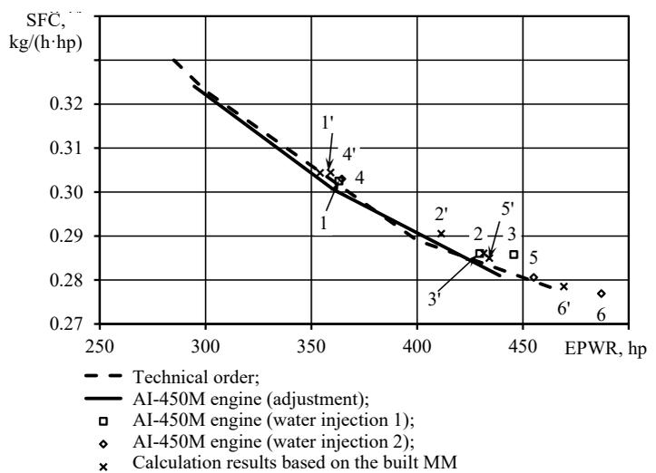
Fig. 4. Change in the specific equivalent fuel consumption (ESFC) depending on engine operating mode and water injection
