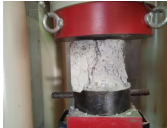
Fig. 1. Testing a concrete cube at the hydraulic press ALPHA 3-3000S
