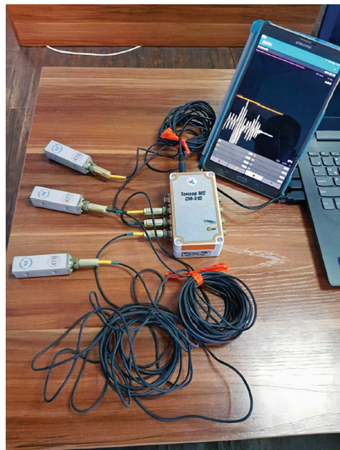
Fig. 4. General view of the measuring complex “Tensor MS”
