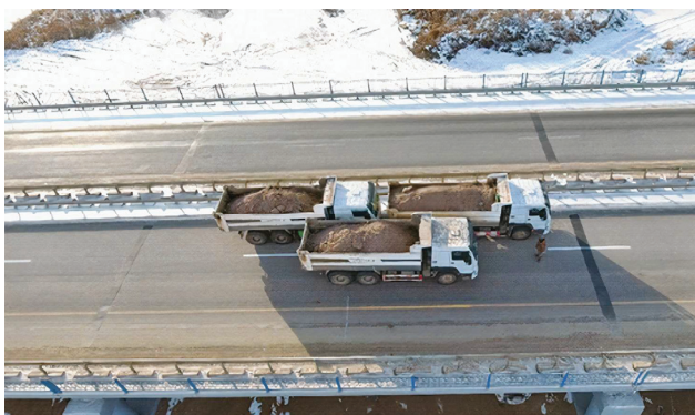
Fig. 2. Scheme of loading the bridge span with test load Case 2. Three trucks are installed on the left side in the direction of travel with a collision with the safety lane
