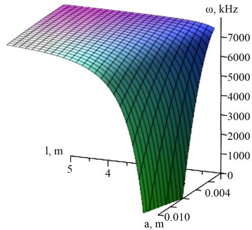
Fig. 4. Dependence of the frequency of longitudinal oscillations on the length of the beam and the initial amplitude at a speed of 5 m/s
