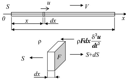
Fig. 1. Diagram of forces acting on a beam element moving along its axis
