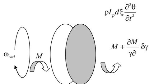
Fig. 2. Diagram of forces acting on the element of the shaft
