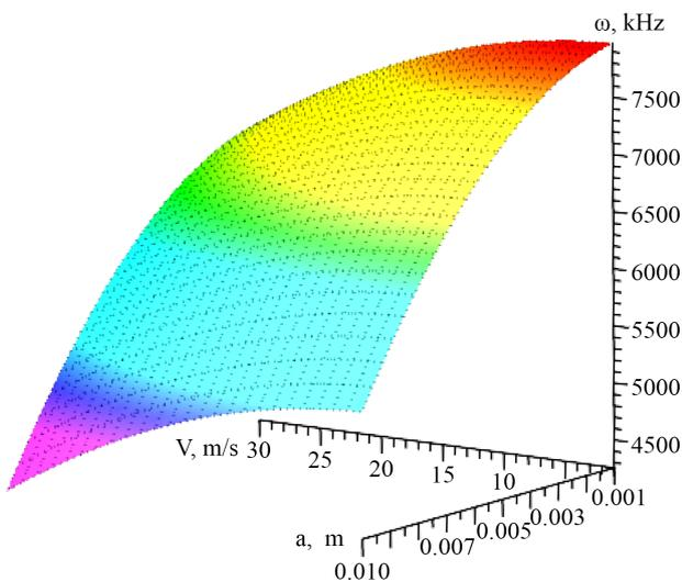
Fig. 3. Dependence of the frequency of oscillation of the system on speed and amplitude
