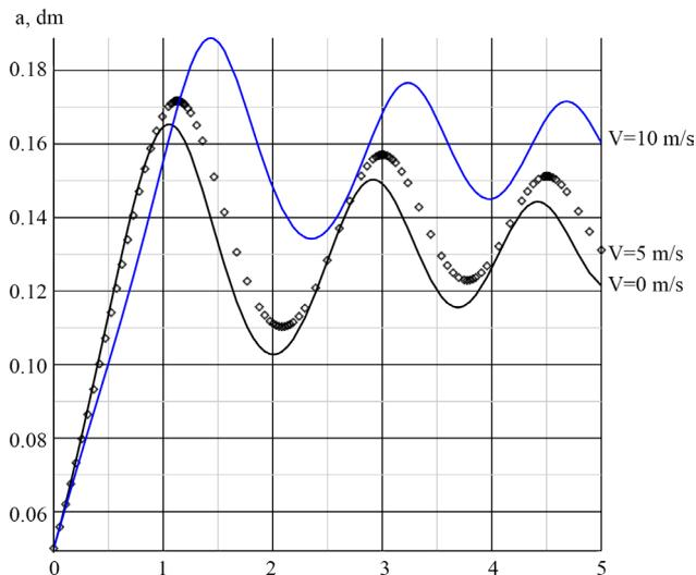
Fig. 6. Transient processes that occur during longitudinal oscillations of the beam for different speeds
