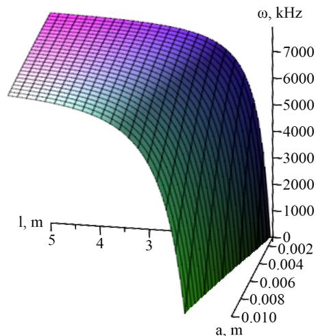
Fig. 5. Dependence of the frequency of longitudinal oscillations on the length of the beam and the initial amplitude at a speed of 20 m/s
