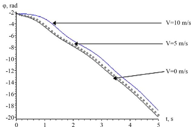
Fig. 7. Dependence of the phase of oscillations of the system for different speeds in a resonant case ( $V=10$  m/s,  $V=5$  m/s,  $V=0$  m/s)
