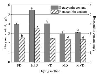
Fig. 4. Betalain content of dried beetroots prepared by different drying methods, different letters indicate significant differences at p<0.05 according to Duncan's multiple test
