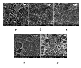
Fig. 3. Microstructure (500× magnification) of dried beetroots prepared by different drying methods: a - FD; b - HPD; c - MD; d - VD; e - MVD
