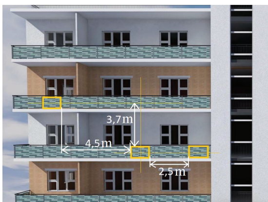
Fig. 9. Diagram with an example of the safe arrangement of external air conditioning units
