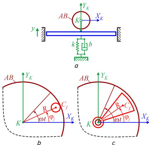
Fig. 1. Single-mass vibratory machine, model, and the kinematics of motion [9]: a – platform; b – ball or roller; c – pendulum
