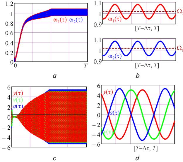
Fig. 3. The onset of the jamming mode  $\Omega_1$  when accelerating the rotor to the speed  $n_0=3.57$ , a slightly lower than the second bifurcation speed  $n_2$ : *a* – plots of changes in the speed of rotation of loads at the interval  $[0, T]$ ; *b* – at the interval  $[T-\Delta\tau, T]$ ; *c* – plots of changes in the motion  $y(\tau)$ , speed  $v(\tau)$ , and acceleration  $a(\tau)$  of the platform at the interval  $[0, T]$ ; *d* – at the interval  $[T-\Delta\tau, T]$
