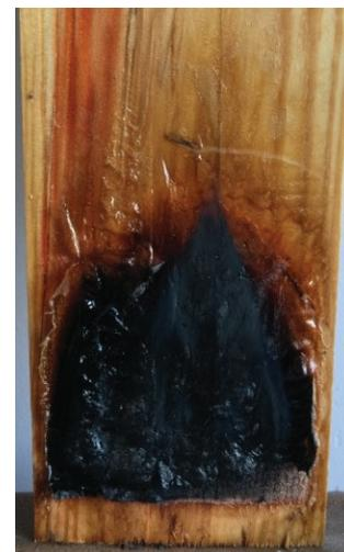
Fig. 6. Swelling of the fire-retardant varnish during thermal action
