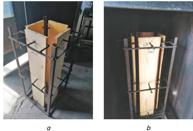
Fig. 5. Samples of wood during combustibility tests: a – before testing; b – after thermal action
