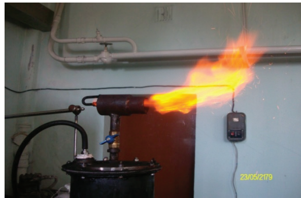
Fig. 10. Photographing the combustion process of coal-water fuel
