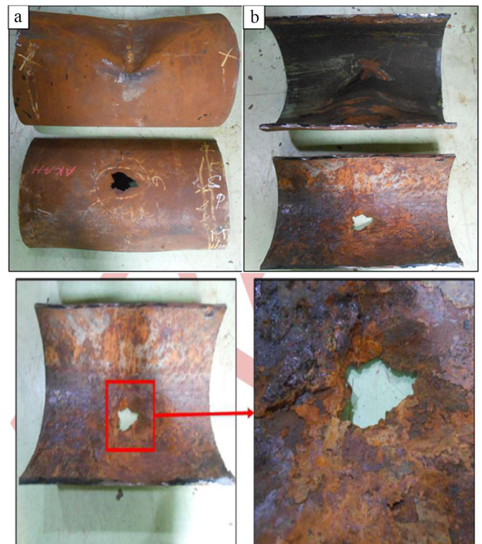
Fig. 2. The specimen of: a – peeled-off coating; b – suspected abrasive affected area
