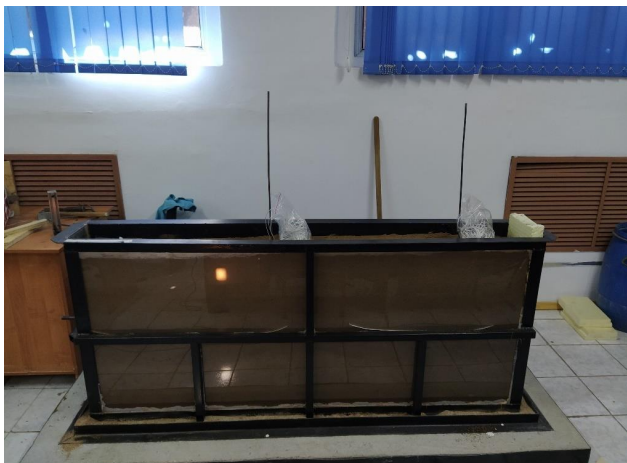
Fig. 2. Geotechnical tray for recording seismic vibrations
