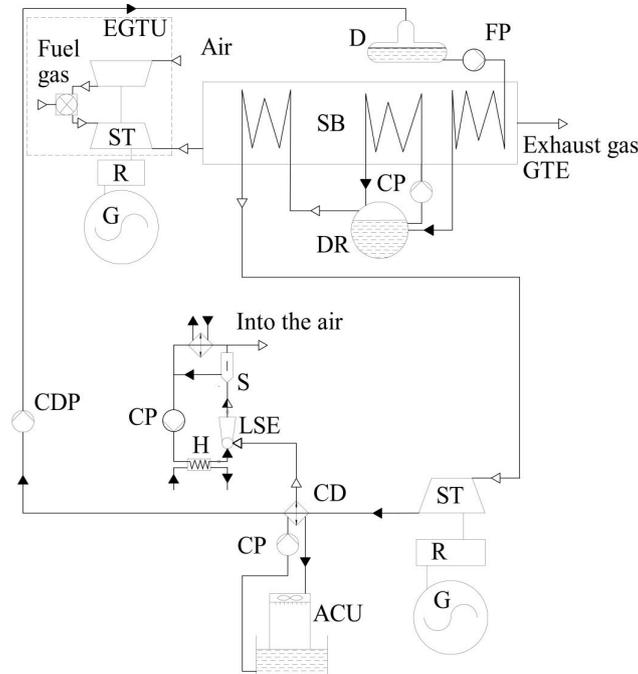
Fig. 3. Alternative scheme of a condensing unit based on a liquid-vapor ejector: LVE – liquid-vapor ejector, S – separator, CP – circulation pump, H – heat exchanger-heater, SB – steam boiler, ST – steam turbine, CD – condenser, CP – circulation pump, CDP – condensing pump, D – deaerator, FP – feed pump, DR – drum, G – generator, R – reducer, EGTU – energy gas turbine unit, ACU – air cooling unit
