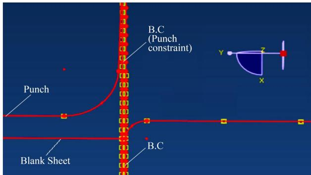
Fig. 12. The applied boundary conditions
