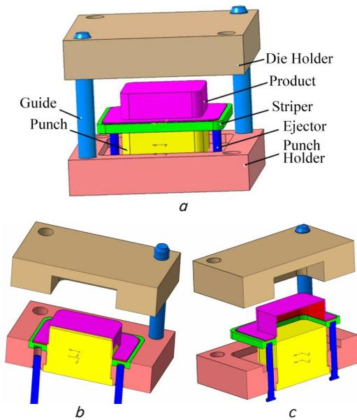
Fig. 8. Modeling the main parts:
