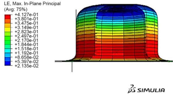
Fig. 17. The contour plot of elastic strain
