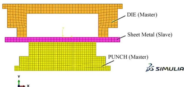
Fig. 9. The main active parts in the simulation process
