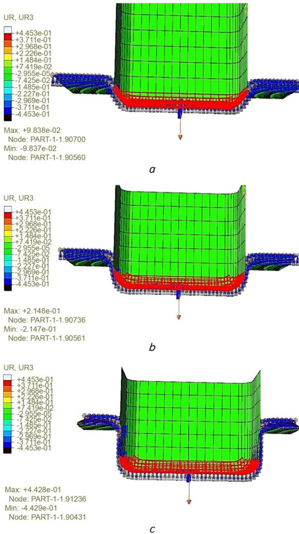
Fig. 15. Punch traveling: *a* – initial movement; *b* – second stage movement; *c* – the final displacement
