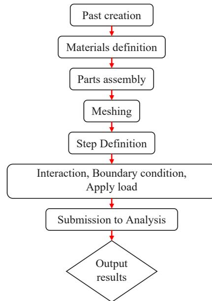
Fig. 10. Flowchart of Analysis process
