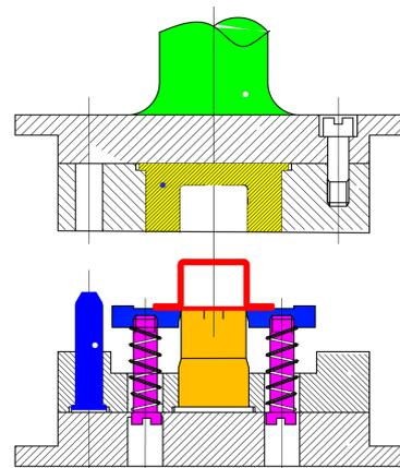
Fig. 7. Part ejection during the final step
