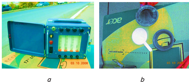
Fig. 3. General view: a – electric aspirator model 822; b – filters, and filter holders
