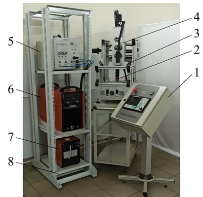
Fig. 8. General view of the set of equipment for welding and determining the residual deformations by the DIC method: 1 – manipulator control panel; 2 – replaceable welding torch; 3 – high-resolution cameras (2 pcs.); 4 – manipulator for performing the welding process; 5 – plasma module; 6 – specialized power supply for TIG and PAW welding; 7 – cooling unit of the welding torch; 8 – equipment rack
