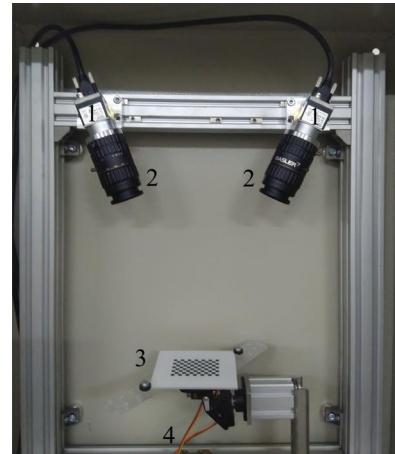
Fig. 1. Laboratory bench for measuring movements by a Stereo DIC method: 1 – digital cameras; 2 – lenses; 3 – calibration plate; 4 – the place of installation of the object under study
