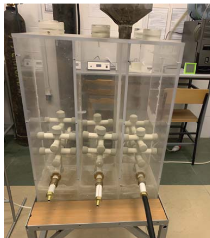
Fig. 2. Laboratory silo-type installation for processing and storage of flour
