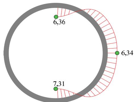
Fig. 6. Deformation distribution diagram in the concrete pipe at the time of destruction
