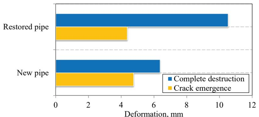
Fig. 9. Results of comparison of the deformed state of pipes at the top of the pipe
