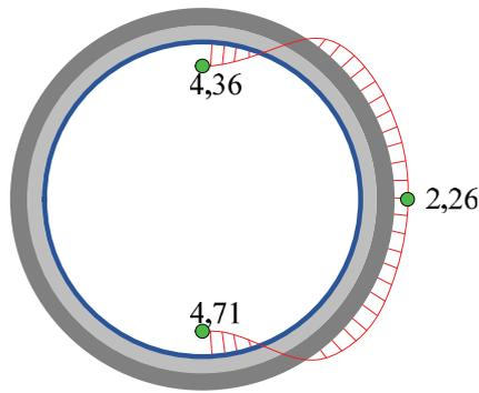
Fig. 7. Deformation distribution diagram in a concrete pipe reinforced by a metal clamp at the time of cracking
