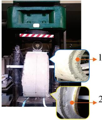
Fig. 3. General view of pipes under study: 1 – pipe without reinforcement; 2 – the pipe is reinforced with a metal clamp
