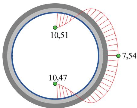
Fig. 8. Deformation distribution diagram in a concrete pipe reinforced by a metal clamp at the time of destruction
