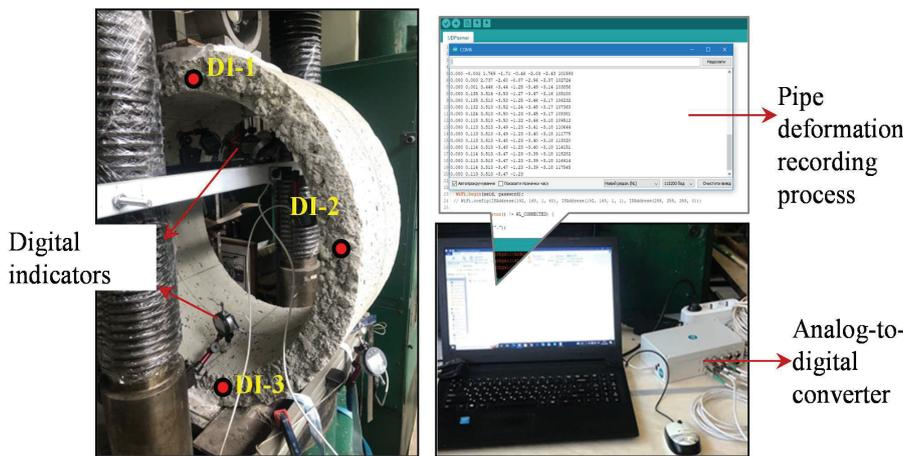
Fig. 4. Experimental scheme of measurements of deflections of reinforced concrete pipe on a hydraulic test press P-250
