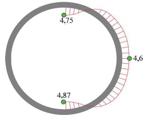
Fig. 5. Deformation distribution diagram in the concrete pipe at the time of cracking
