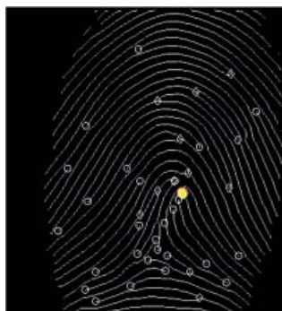
Fig. 7. Representation of Core Point, Bifurcations and Terminations
