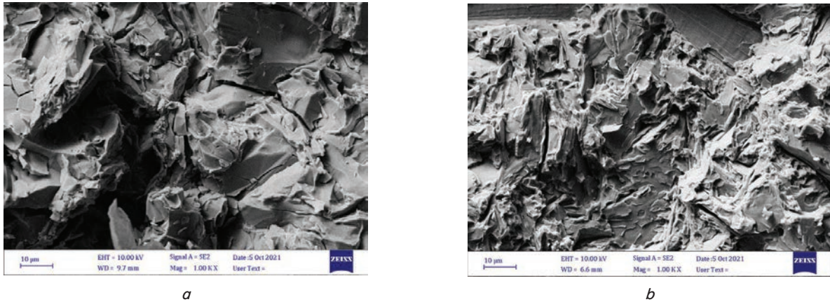
Fig. 16. Field Emission Scanning Electron Microscopy Morphology for fracture section: a – 2 % alumina sand casting; b – 2 % alumina metal mold casting
