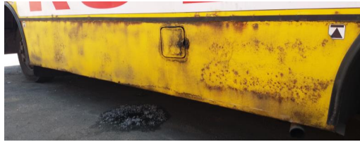
Fig. 5. Bus «Bogdan» A092 with corrosion damage to the body cladding
