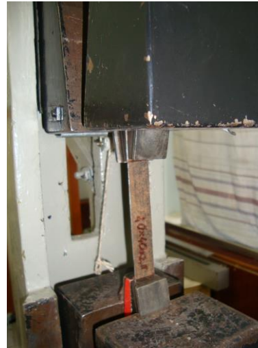
Fig. 12. Testing samples of body frame elements on the breaking machine R-5 according to ISO 6892-1:2019
