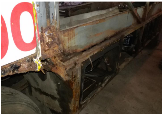
Fig. 6. Corrosion damage to the body under the cladding of the city bus «Bogdan» A092
