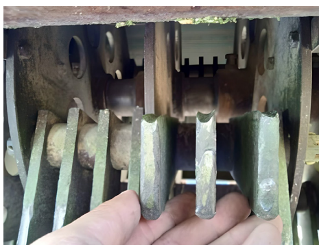
Fig. 5. General view of the location of the hammers on the rotor
