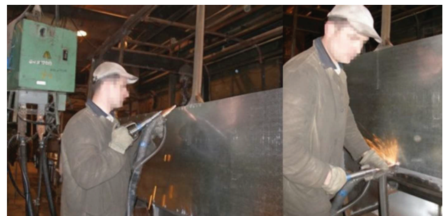
Fig. 3. Manual contact spot welding of the bus body
