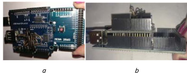
Fig. 1. Arduino Mega board with Shield card reader to protect against BadUSB vulnerability: a – top view; b – side view
