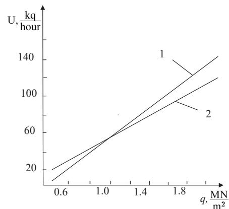
Fig. 1. Dependence of the productivity of the roller gin on the average pressure of the knife pressing: 1 – corresponds to the fine-fiber raw cotton of the variety 5904-I of the 1<sup>st</sup> grade, manual collection, fiber type III; 2 – corresponds to the variety C-6029 of the I-th grade, manual collection, fiber type I)
