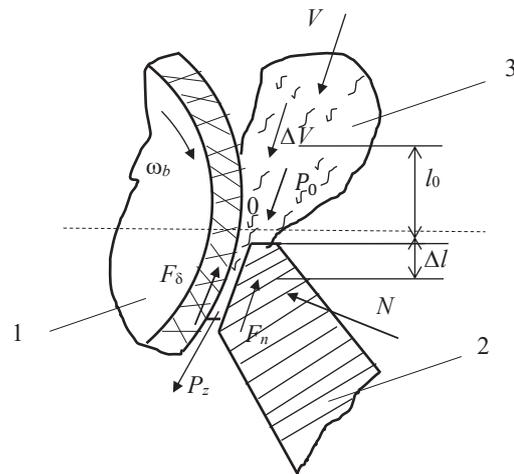
Fig. 2. Scheme of interaction of the knife with the drum: 1 – drum; 2 – knife; 3 – flyer, at  $V > \omega_b$ ;  $V < \omega_b$  when  $\Delta V = 0$ ,  $P = P_0$ ,  $\Delta l = \Delta l_{max}$
