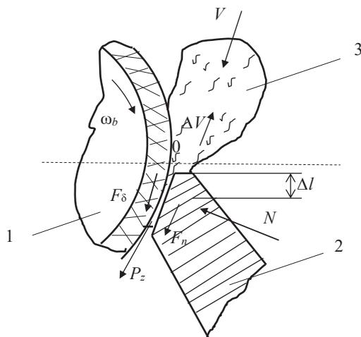
Fig. 3. The balance of power at the end of the push when  $P_0=0, \Delta l \neq 0, l_0=0$
