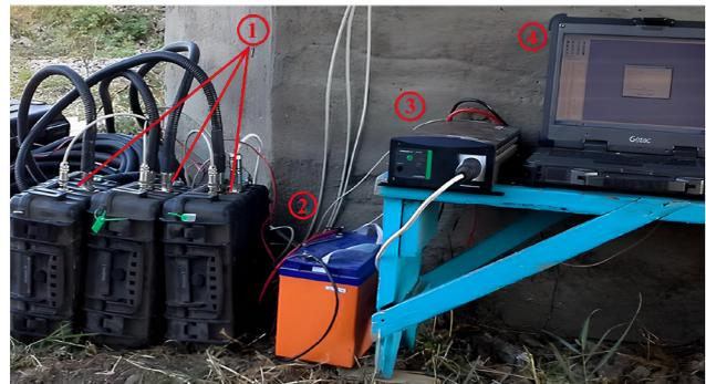
Fig. 4. Mobile complex general view for strain gauge measurements: 1 – measuring modules; 2 – storage battery; 3 – sine inverter; 4 – semi-industrial computer
