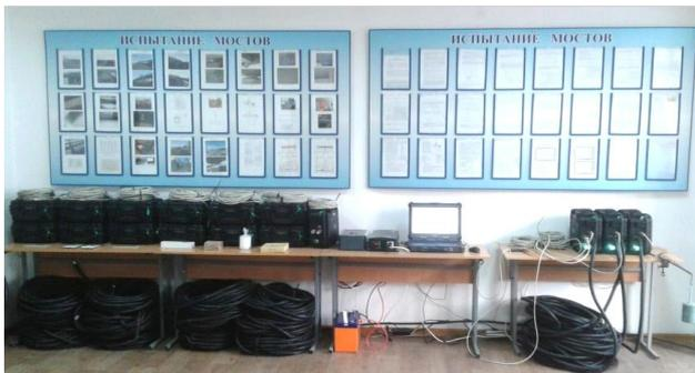
Fig. 1. Strain measuring and computing complex for measuring relative deformations and stresses in structures
