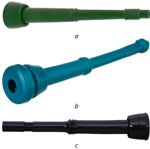
Fig. 1. Samples of teat rubbers submitted for research: a – rubber BARBAROS Liner 8S green from food grade silicone material (France) – sample No. 1; b – rubber IQ Pro elongated from food silicone material (Germany) – sample No. 2; c – rubber Melasty 3111 from material rubber (Turkey) – sample No. 3
